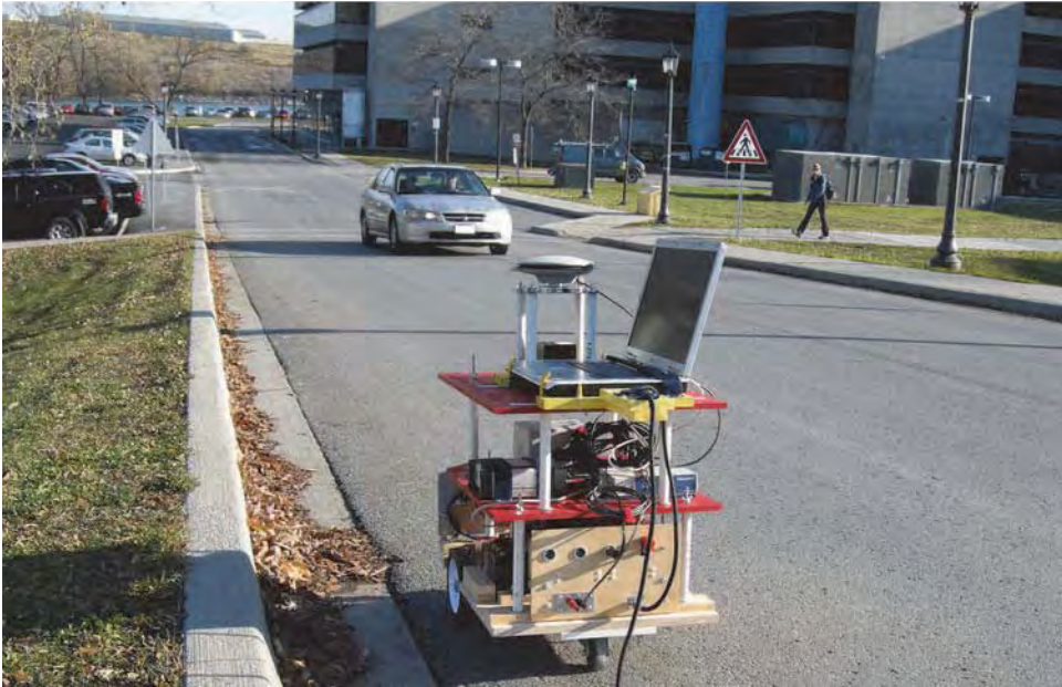
Fig. 2. The mobile robot used for the experiments in this work, custom-built by the author and members of the Electrical and Computer Engineering Department at Royal Military College of Canada.
