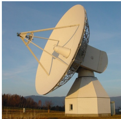
Figure 2. The RTW (Radio Telescope Wettzell), a 20m diameter geodetic VLBI antenna at the Geodetic Observatory Wettzell, Germany (BKG/FESG), has observed the largest number of observations within IVS campaigns
