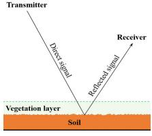
Figure 3. Bistatic radar geometry of spaceborne GNSS-R remote sensing soil detection.
