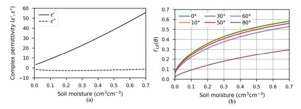
**Figure 2.** Complex permittivity under different soil moisture (**a**) and the relationship between soil moisture and reflectivity at the different signal incidence angle (**b**).
