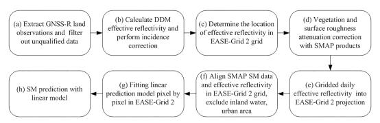
Figure 4. Spaceborne GNSS-R SSM retrieval algorithm flow chart.
