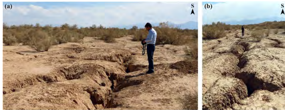
Figure 9. Photograph looking South taken from the location of the red circle on Figure 8a which illustrates the fissures that have developed as a result of the observed differential subsidence (the person shows the scale).
